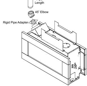
When using Rigid Vent other than Simpson Dura-Vent, 3 screws must be used to secure rigid pipe to adaptor.
