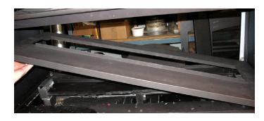
5) Remove burner by removing 2 screws.
