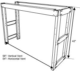
3. If installing the unit with horizontal venting—secure the 2 (two) top horizon studs using the inner holes—cut the remainder of the stud (repeat at oth end) before proceeding to Step 3.
