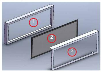
Remove screws from inner side of the inner door trim and discard screws and the brackets. (Brackets not shown). Remove the screen mesh from inner door trim.
