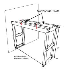
5. Install the 2 long horizontal studs(Top:588-019; Bottom:588-022), secure with 2 screws on each end - if installing with horizontal vent exit see Step 4 before installing.
