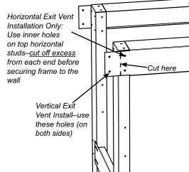
4. Install 2 top horizontal studs (588-024) with 2 screws on each side.
