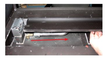
7) Remove 7 screws to remove left access panel .
