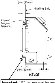
**Important:** 1/2" gap required between faceplate and finished wall.
