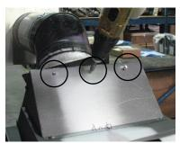
3) Install the deflector near the vent outlet - secure with the same 3 screws. Ensure flange on deflector is facing downward.
