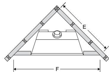
Note: If this is an outside corner, the minimum distance between the vent and the outside corner is 6" (15cm) with AstroCap termination cap or 12" (30cm) with Rigid Vent termination cap. (For example Dura-Vent)
