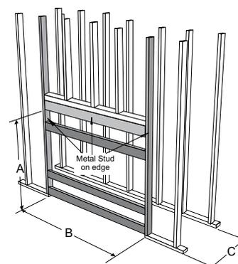
**Note:** Three horizontal steel studs must be installed after the unit is in position and the venting, gas and electrical is installed. The horizontal studs allow the non-combustible wall board to be attached and supported.
